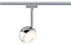
Spot Capsule II URail Spot incl. 1×6,3W 439lm, 2.700K ↖ 30° 230V ⌀210 ⇄80 ↗80 mm 95455
